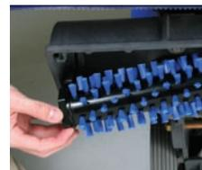
The 16 or 18 inch scrub brush can be removed and installed without the use of tools.
