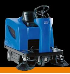
FLOORTEC R 670 series includes a battery (B) and a petrol (P) model, both available with 700 mm main broom. In case you want to add extra equipment to match specific cleaning needs, we provide a wide selection of options to choose from.
