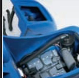
The recovery tank can easily be removed and clean away from the machine and it also permit full access to battery compartment.
