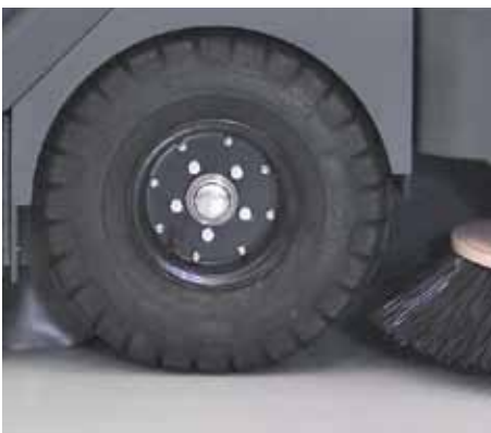
The large wheels give a smoother ride and allow the machine to mount kerbs without difficulty
