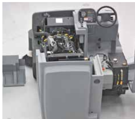
Exceptionally easy serviceability is achieved with Nilfisk's NoTools™ system. The 5-sided access to engine and hydraulic components saves time and keep down the service cost
