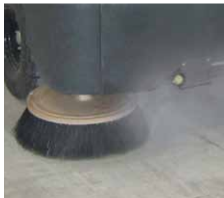
The exclusive DustGuard™ system effectively controls airborne dust by providing a fine mist of moisture to the front and side brushes
