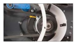
Fully controllable clutch - eliminates problems with marking the floor on start-up
