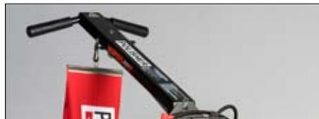
The ergonomically designed handle is adjustable and is fitted with a throttle control - right at the Operator's fingertips. It can also be folded down for easy transport.
