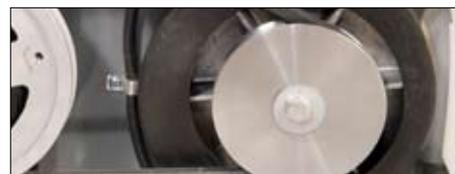
The skirt is positioned within the machine body for greater protection as well as containing the dust so that the active vacuum system leaves the floor dust-free.
