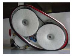
Counter-rotating 'Jackaroo' pads, combined with the 'flexible' pad holder and pulley system means both pads constantly follow the contours of the floor – giving an exceptionally smooth and even finish.
