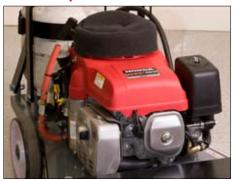
A 12 volt push-button start, fires the 13hp (9.69 kw), 4 stroke overhead valve Honda engine into action while the brushes are on the floor.
