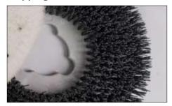
Three quick-release Tynex abrasive brushes, rotating between 350 and 700 rpm, easily strip a 51cm width.
