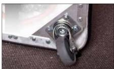
Four omnidirectional castors makes moving the machine on the job or transporting, smooth and easy. With one lockable wheel as a brake, 'Terminator' is 100% stable as well as easy to use ...and move.
